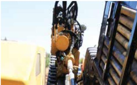
**DUAL ROD TECHNOLOGY.** Contractors can meet the challenges of their jobsite with Vermeer dual rod technology. Using a dual threaded joint, the inner rod provides torque to the drill head, while the outer rod offers steering capability to the drill head and additional rotational torque.
